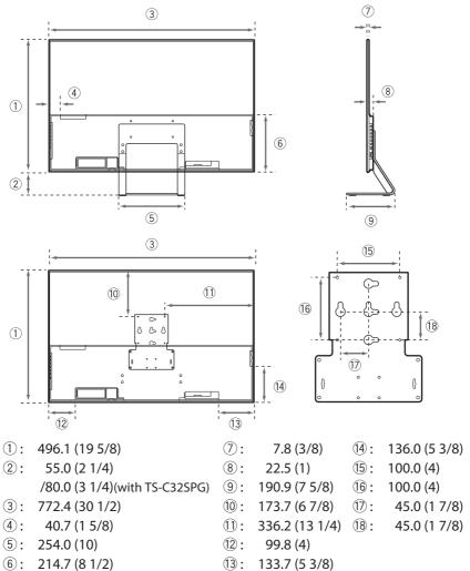
Use screws of adequate length (M4 × 12 – 16) to fix the VESA bracket and wall mount adapter.
